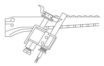
Fig. 34: Pilot Burner Flame (Standing Pilot Units)
